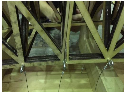
Figure 4: Visible shearing at joint corresponding to Q in diagram.
