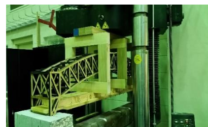
Figure 3: The model under the Satec ULM, prepared for load testing
